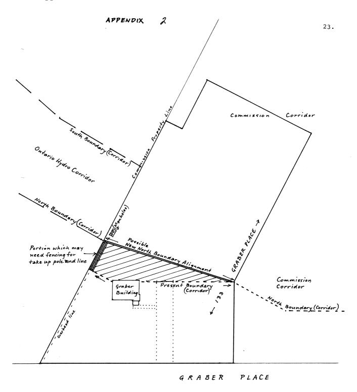
SHADED PART: With the dog leg eliminated in northern route of high tension lines, a new alignment of the northern boundary of the corridor would add shaded part to that portion of 133 Graber Place outside of the corridor. a parcel with potential for severance.
